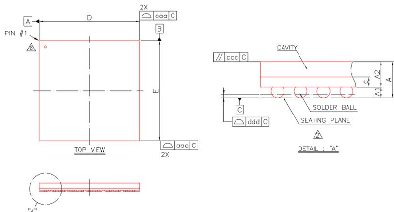
Fig.2-6 RK3308GK Package Top View and Side View
