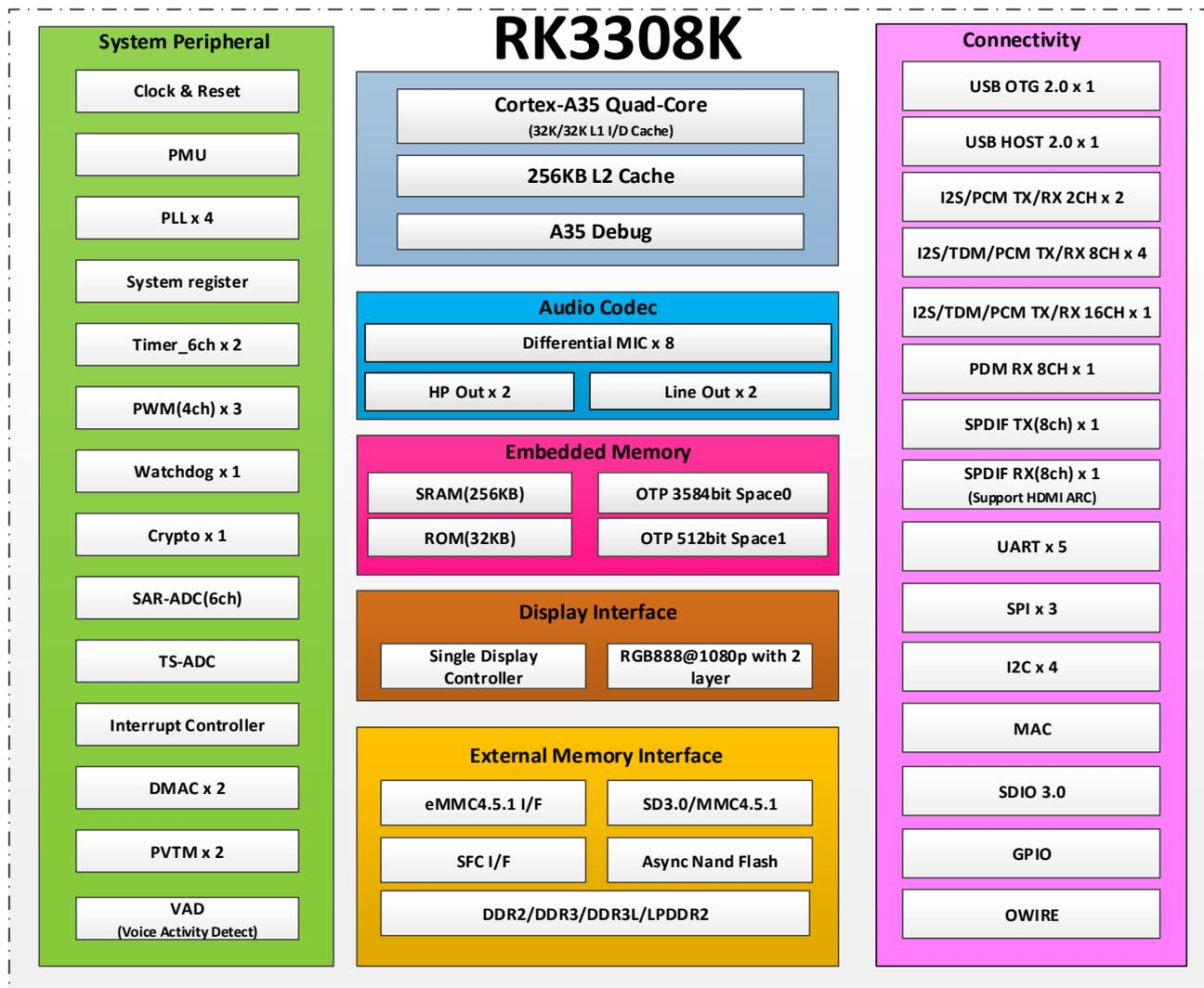
Fig.1-1 RK3308K Block Diagram
