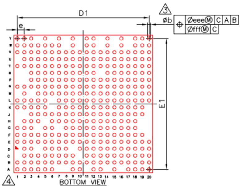
Fig.2-4 RK3308K Package bottom view
