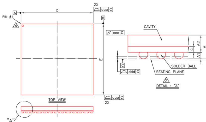
Fig.2-3 RK3308K Package Top View and Side View
