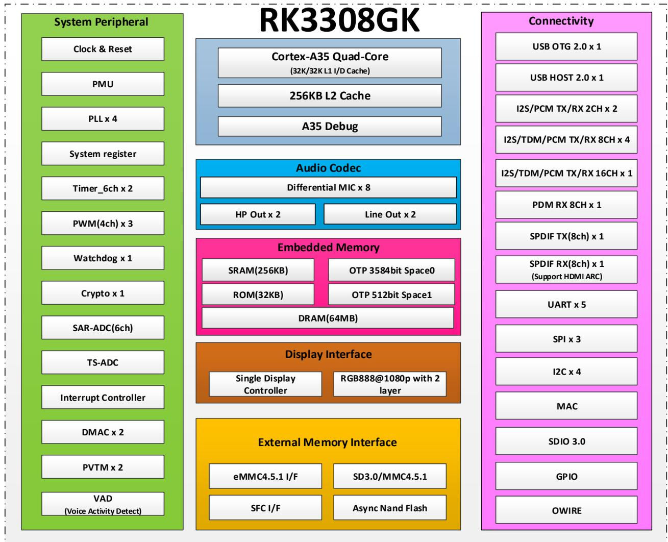
Fig.1-2 RK3308GK Block Diagram
